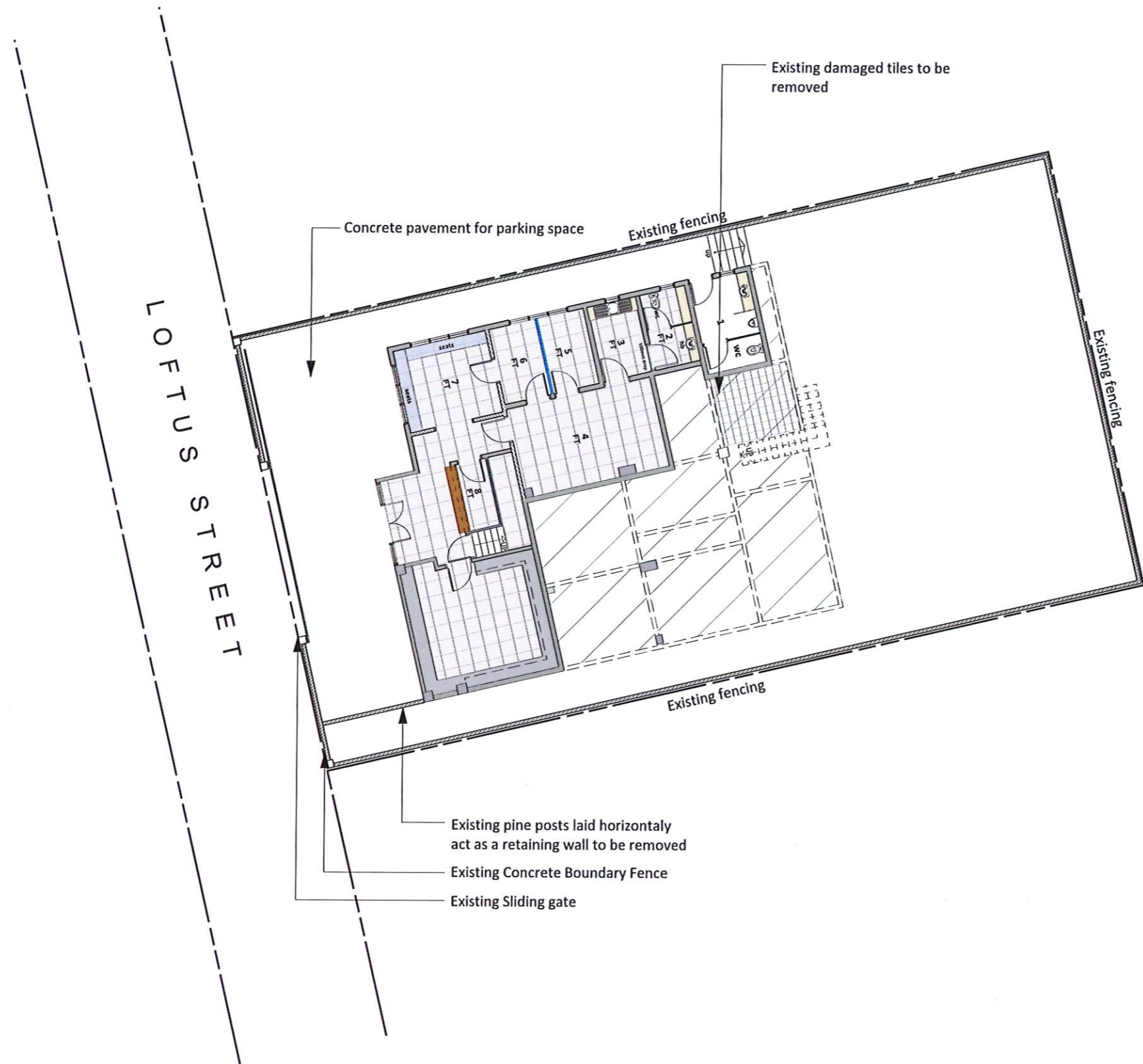
EXISTING SITE PLAN Scale 1:200 @ A3.
