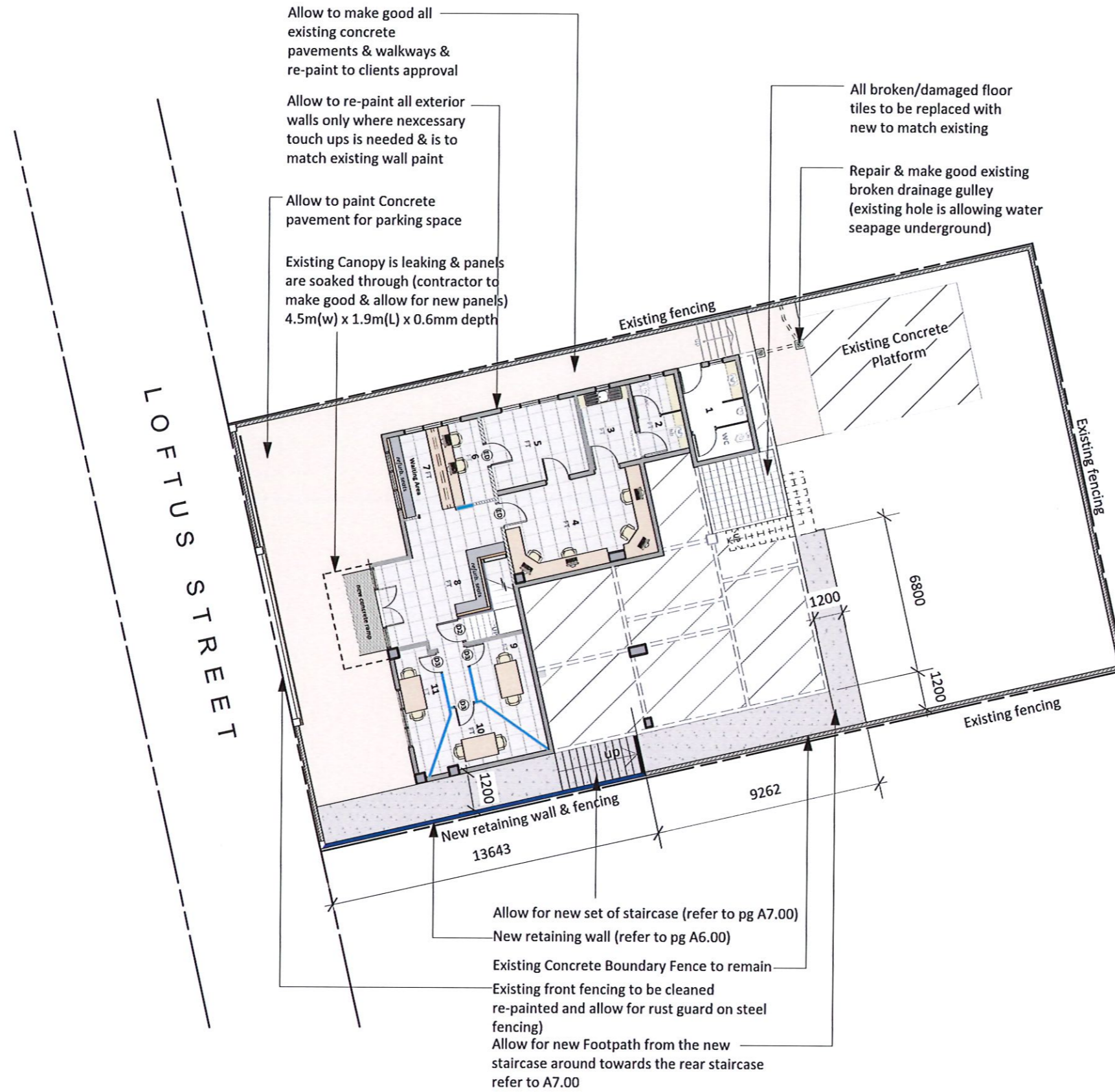
PROPOSED SITE PLAN Scale 1:200 @ A3.
